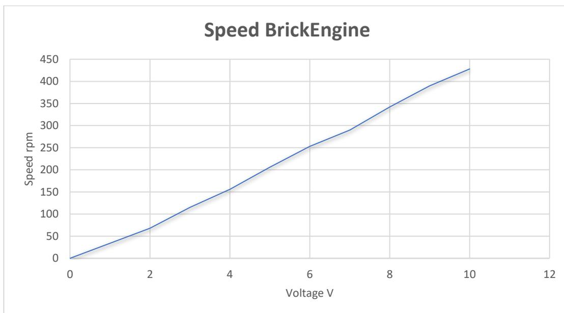
Fig 11: Speed diagram Brickengine V1
