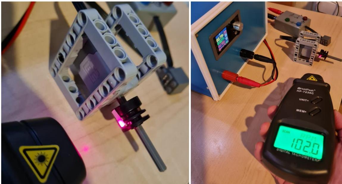
Fig 31: Reflectors on rim and measurement
