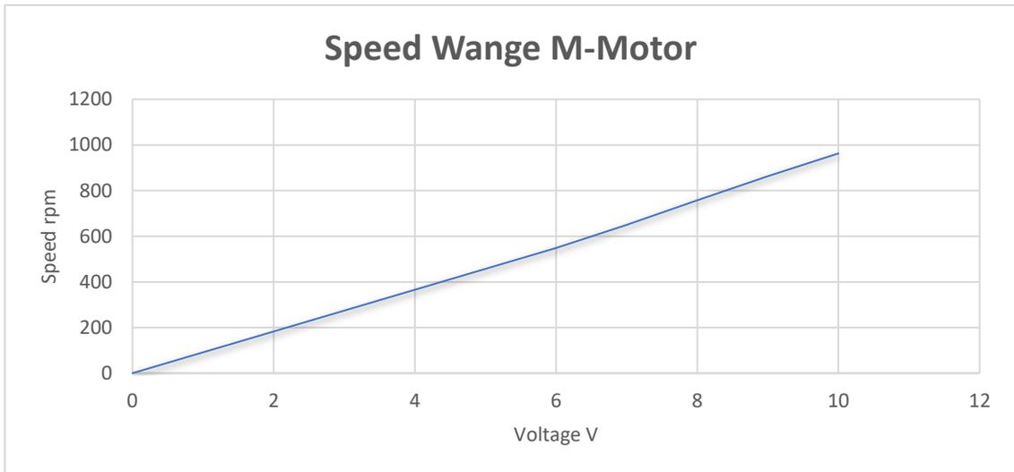
Fig 27: Speed diagram of Wange M-Motor
