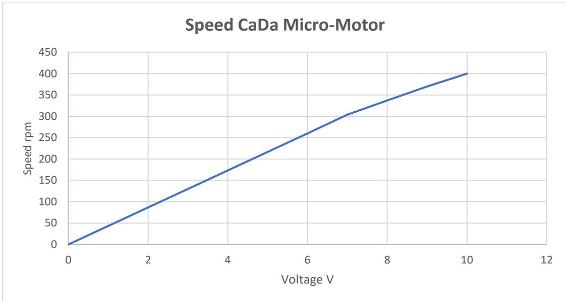
Fig 24: Speed diagram of CADA Micro motor
