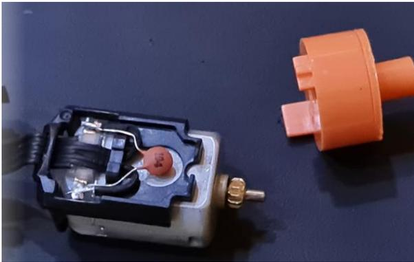
Fig 3: Blue Brixx L-Motor Interior
