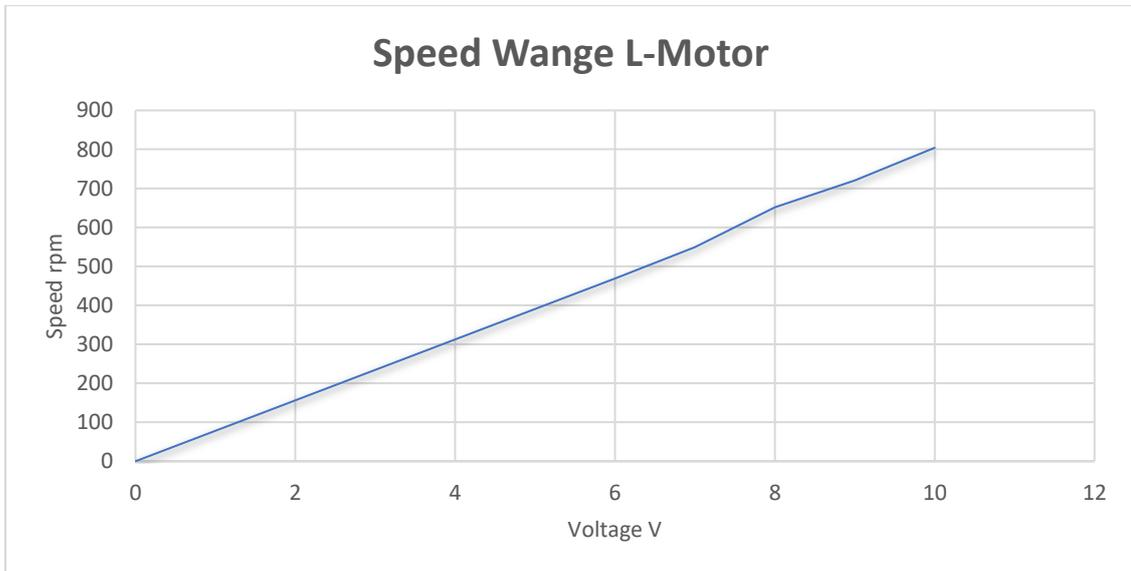
Fig 28: Speed diagram of Wange L-Motor
