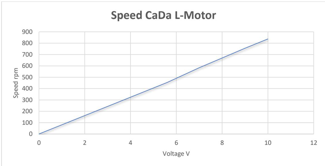
Fig 20: Speed diagram of CADA L-Motor
