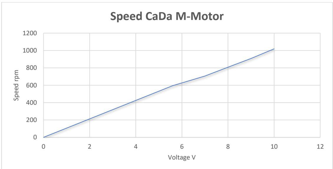
Fig 21: Speed diagram of CADA M-Motor
