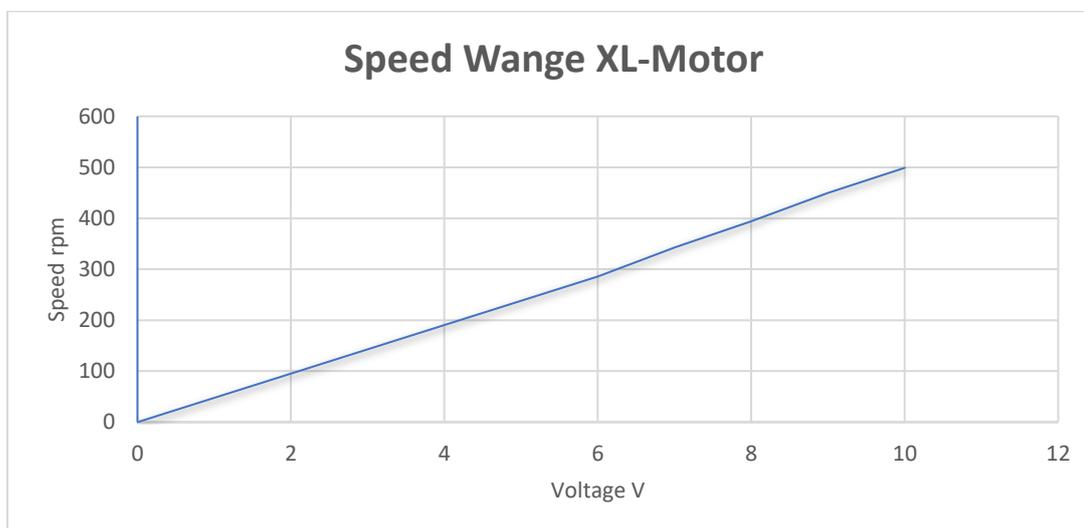
Fig 29: Speed diagram of Wange XL-Motor
