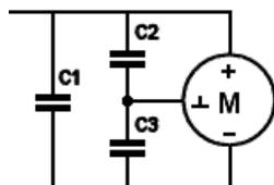
Fig 1: Interference suppression of a DC motor with capacitors
