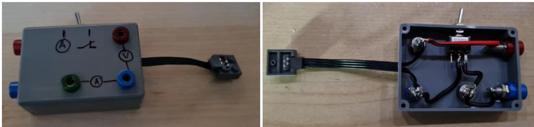
Fig 30: Measuring box for Power Functions motors
