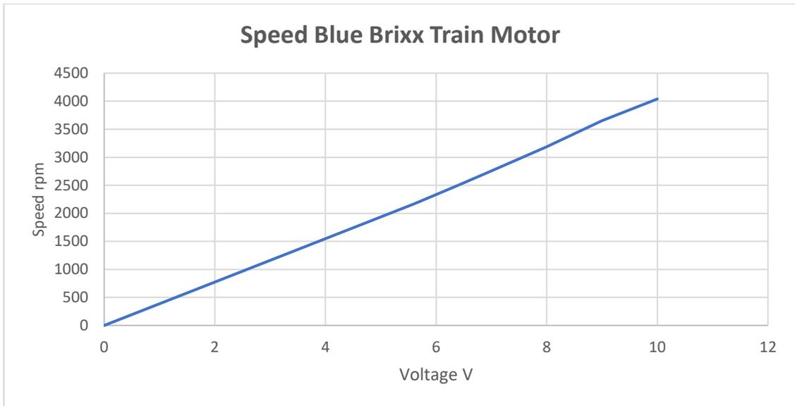
Fig 8: Speed diagram Blue Brixx Train Motor
