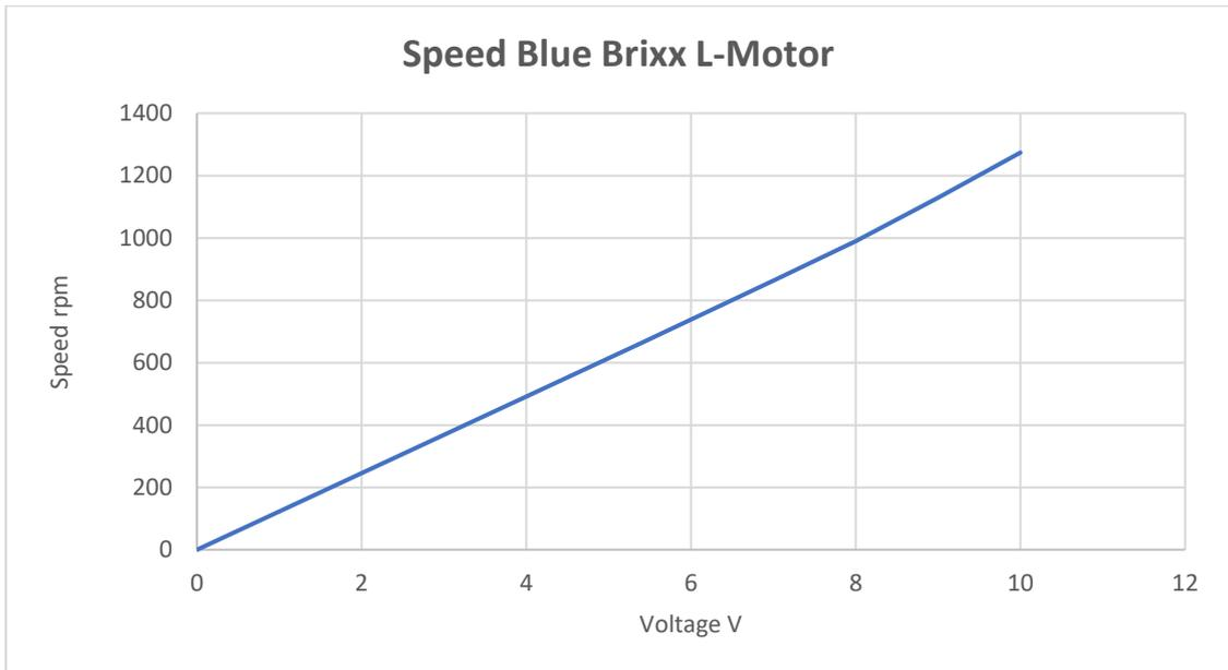
Fig 6: Speed diagram Blue Brixx L-Motor
