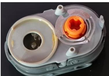
Fig 17: Gear and contact plate of the angle encoder
