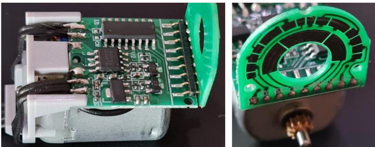
Fig 16: Control electronics (left) and angle encoder (right) of the CaDa servo
