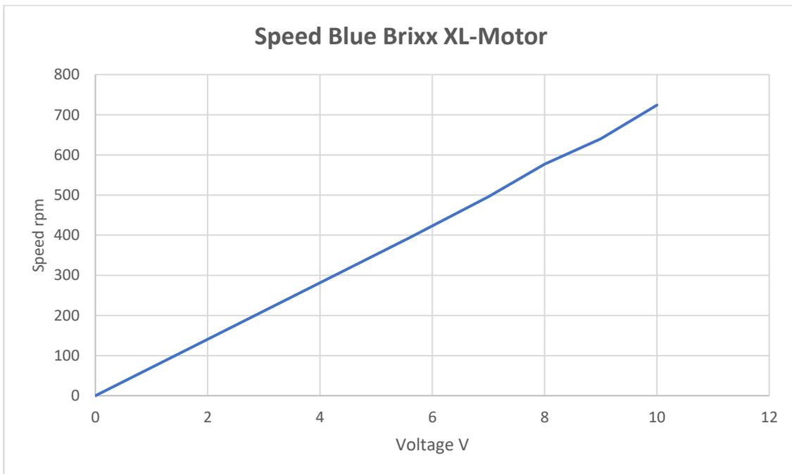
Fig 7: Speed diagram Blue Brixx XL-Motor
