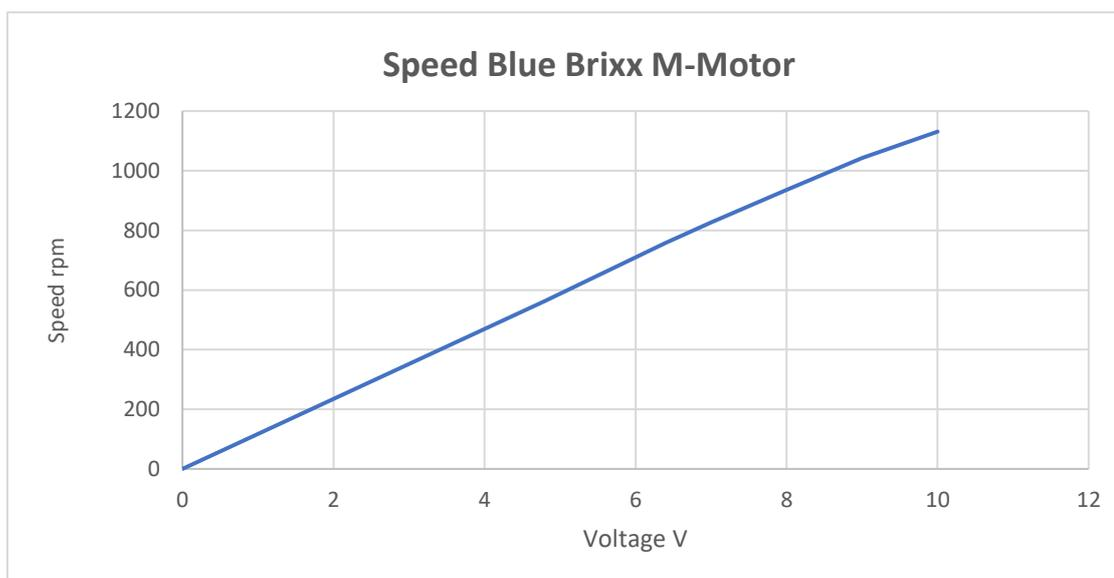
Fig 5: Speed diagram Blue Brixx M-Motor
