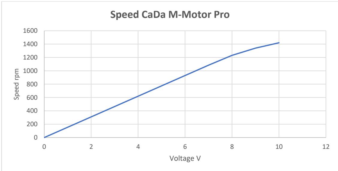
Fig 23: Speed diagram of CADA M-Motor Pro
